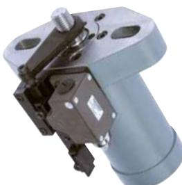
**Hydraulic cylinder with attached limit switch operation**
